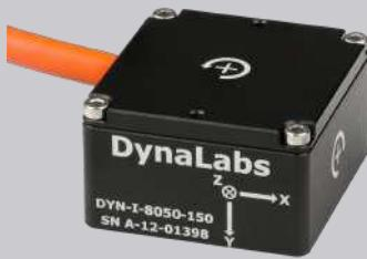
Dynalabs IMUs enable separate analog voltage outputs for all 6 degrees of freedom(DOF). IMUs enable power supply voltage from 6 to 35 VDC. Dynalabs IMUs feature a lightweight, reliable aluminum housing with protection class IP68 and have cable with configurable length and connectors.
